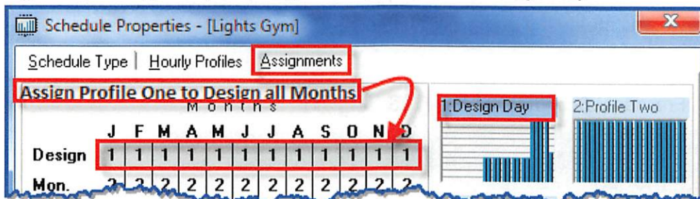
Figure 1.15 – Lights Gym - Assign Hourly Profile 1 to Design Day
