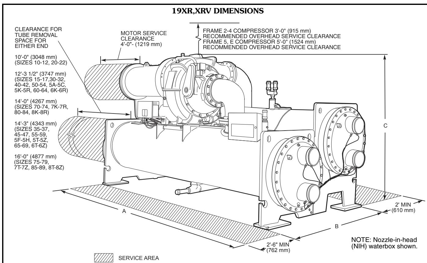
**19XR,XRV DIMENSIONS — SINGLE-STAGE COMPRESSOR AND TWO-STAGE COMPRESSOR FRAME SIZE E (Marine Waterbox)**
